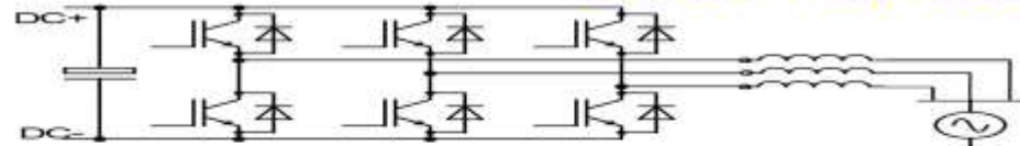
Config. 1: IGBT-based voltage source converter (VSC-IGBT)
