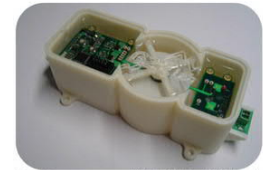
DC-DC converter (15V-5W) with insulation voltage capabilities up to 40kV (Schneider)
