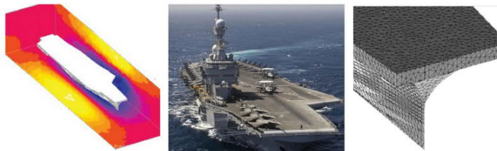
Magnetic State of a aircraft carrier in a earth magnetic field (FLUX software)
