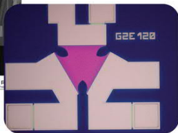
Hybrid transducers for voltage controlled actuation piezoelectric / magnetostrictive multilayers (@ CEA-LETI)
