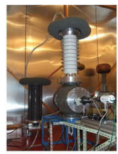
HVDC 350 kV test cell for the measurement of dark currents through pressurized gases
