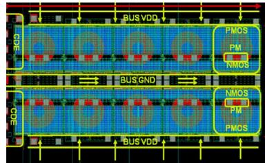
Layout of the 5V 2A Elementary Cell power die. Based on a standard technology this die offers a low cost and high efficiency active part to the Elementary Cell
