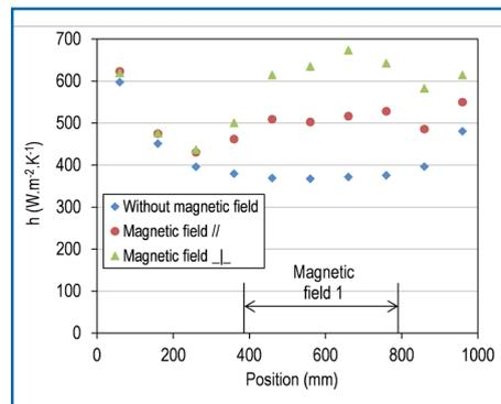
Figure 2: Improvement of the convective heat transfer coefficient in a square duct. Influence of the direction of the magnetic fluid.
