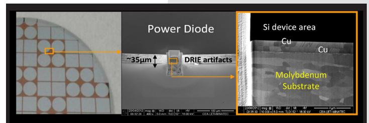
Zoom into the bonding region between a vertical power diode and the metal substrate (Left: photograph, center and right: SEM).
