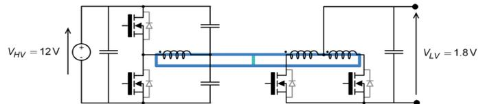
Resonant converter 12V/1.8V, 1W, 2MHz
