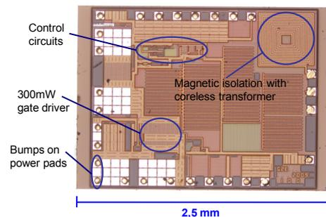
Example of a dedicated CMOS driver including gate signal insulation, driver self supply and power gate charge control
