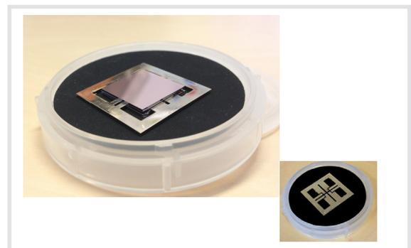
Dummy 3D assembly of matrices of vertical power transistors and vertical power diodes. Inset: Zoom on the electrical interconnection frame
