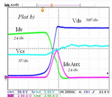
Energy storage during power device switching transitions
