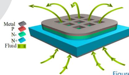
Figure 1: Integration of cooling channels perpendicular the PN junction in a power chip
