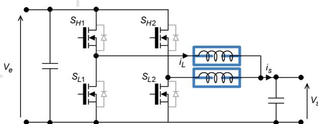
Interleaved Buck converter 12V/3.3V, 10W, 2MHz
