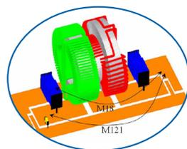
Modeling of an EMC filter including all stray couplings with components and PCB tracks. InCa 3D ® model. Different layouts comparison.
