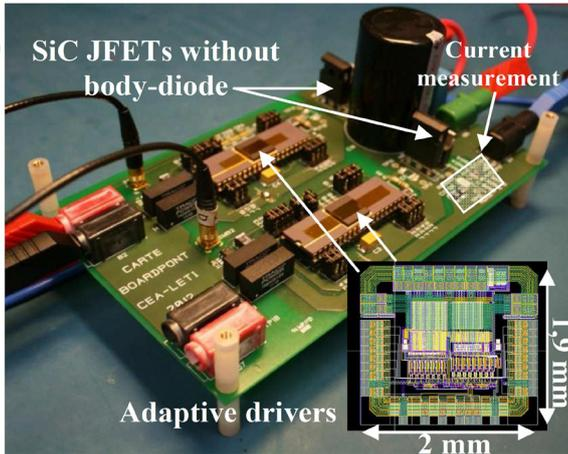
Dedicated driver for wide band gap power devices, including adaptive output stage
