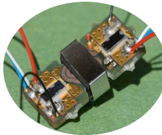
10W-10kW/Liter Elementary Cell based on Dual Active Bridge structure using 2 power dies flip-chipped on a PCB including a planar transformer
