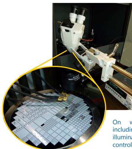
On wafer characterization, including variable optical illumination and temperature control
