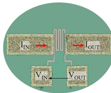
Figure 3: Thermal sensor integrated on the surface of a power diode
