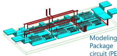
Modeling of a Power Electronics Package including the gate circuit (PEEC Method in InCa3D ®)
