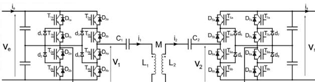
DC/DC series-series resonant converter for Electric Vehicle battery charger (20kW)
