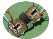
10W-10kW/Liter Elementary Cell based on Dual Active Bridge structure using 2 power dies flip -chiped on a PCB including a planar transformer
