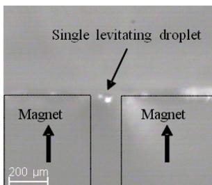
Levitation of 30 μm water micro-droplets over millimetre-sized NdFeB magnets
