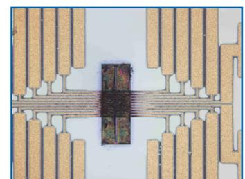
MEMS combining diamagnetic levitation and dielectrophoretic manipulation
