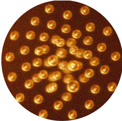
Top : Diamagnetic levitation of micro-droplets of water, mutually repulsed by their electrostatic charges.
