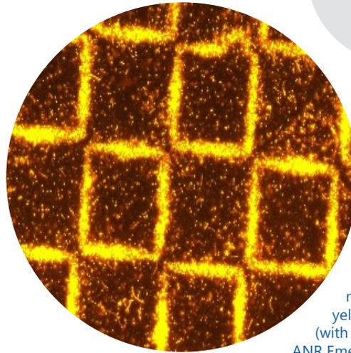
Magnetically-tagged bacteria trapped above an array of micro-magnets. Flat 50x50 μm magnetic grid obtained by thermo-patterning. Bacteria having internalized superparamagnetic nanoparticles. Detection by yellow fluorescence. (with Ampère/ECL, Institut Néel - ANR Emergent)
