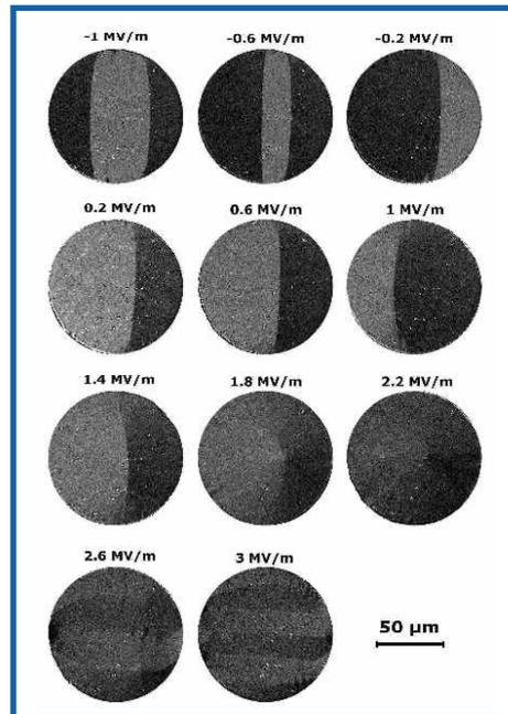
Direct magneto-optical Kerr observation of the rotation of the easy axis in 100 μm circular pods, for increasing values of the electric field applied to the demagnetized composite.
