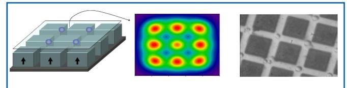
Matrix of microparticles in diamagnetic levitation / confinement in a paramagnetic buffer solution. Left: Principle, Centre: Simulated magnetic traps, Right: Matrixed yeast cells (with LETI/CEA, Ampère/ECL)
