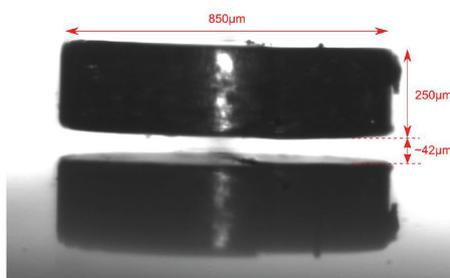
Fig.2 : double-dipole miniature magnet (phi 850 μm) in stable levitation 15 μm above polished graphite. The twin-magnet structure is visible in the reflection.
