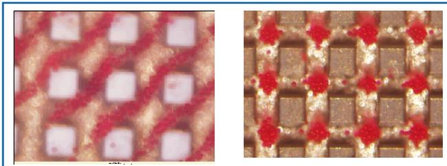
Diamagnetic latex beads (red) guided and matrixed above topographically patterned micro-magnet arrays (with Néel, Biopuces, LMGP)
