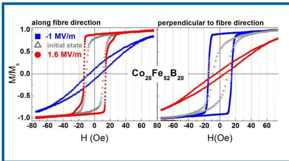
Normalized magnetic hysteresis cycles switched by applying opposite electrical fields, and measured along the fibres (easy axis) and perpendicular to the fibres (hard axis).
