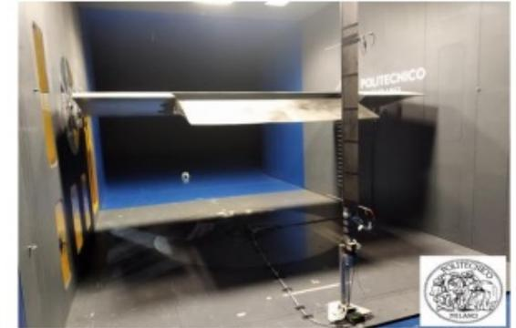
Large-Scale A320 SMS prototype (near scale 1) in the wind tunnel of POLIMI
