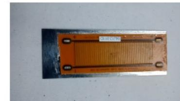
(a) Comercially available piezoelectric fiber composite
