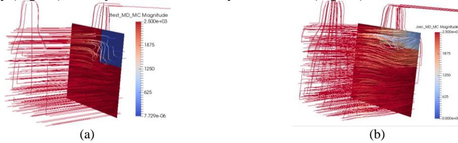
Fig. 2 Experimental results – Stack simulator: Real current (a), Identified current from magnetic field (b)
