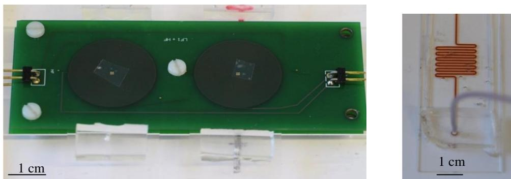
Fig.1 (a) Realized PCB sandwich structure that includes excitation coils (HF and LF) and sensors; (b) Realized microfluidic reservoir
